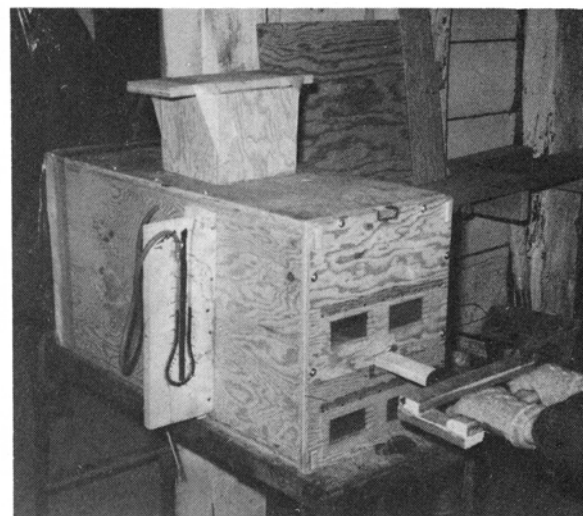
Fig. 5. Front End of the Durability Test Pump, showing the lower fixed part (below piston rod) and the upper removable part, that is held by 6 screws with flat washers. Felt weather-stripping makes the removable part airtight.
