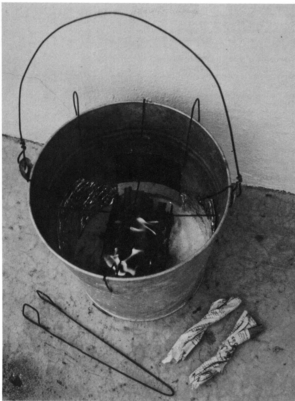
Fig. 9.3. Bucket-stove with its sliding damper partly closed. Foot-long tongs of coat hanger wire are especially useful when burning twisted half-pages of newspaper.
