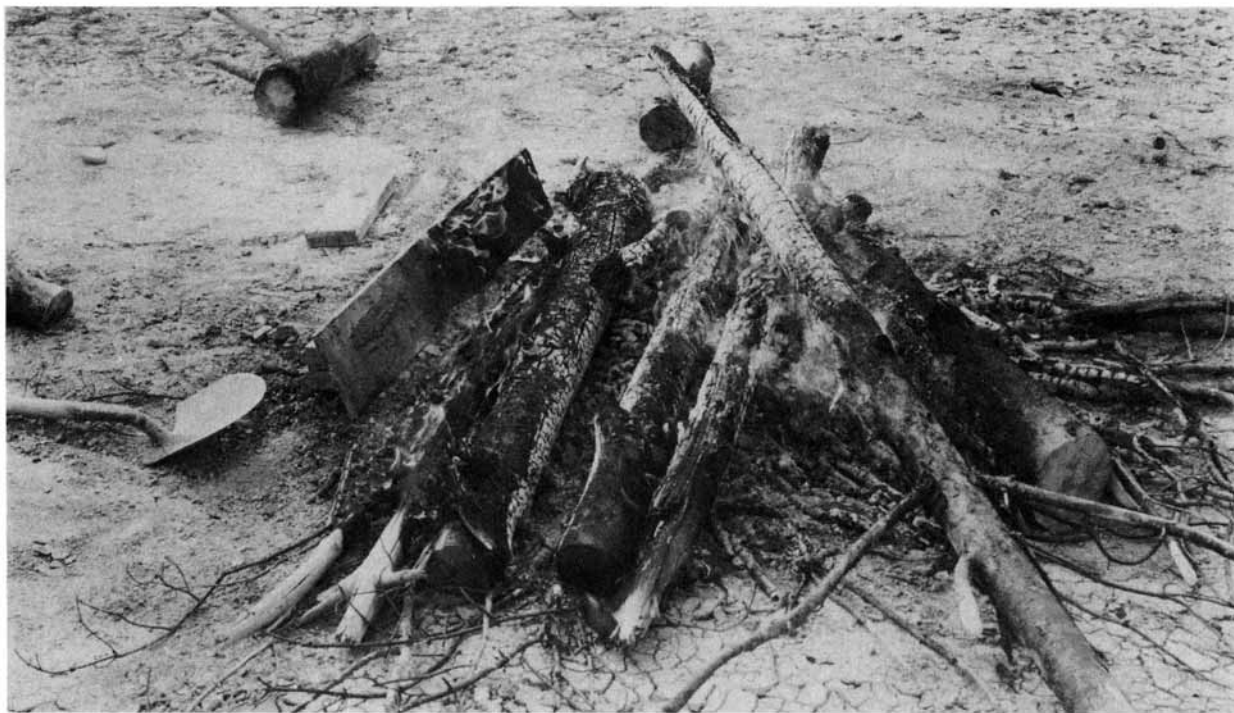
Fig. 7.3. Heat radiation had ignited the flaming half of the board on the ground, while the half near the shovel—painted white with a thick coating of slaked lime—had not even begun to smoke.
