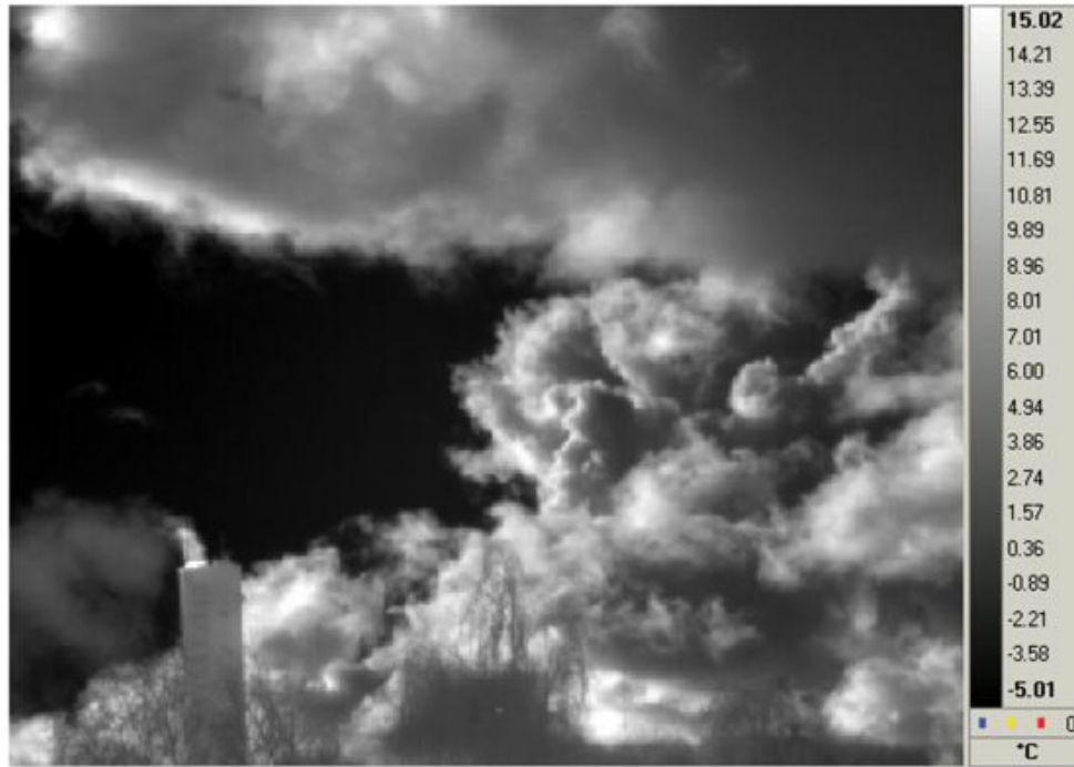
Fig. 10.6 IR image, obtained in the wavelength range 9–12 \mu\text{m} . Ground temperature, approximately 0 °C. Smokestack and treetops are visible at bottom. On the temperature scale provided by the camera manufacturer, distant cloud regions register hotter than 15 °C despite a surrounding air temperature of minus 20 °C. Thus, the temperature scale paradoxically implies a sustained temperature gradient of 35 °C.
