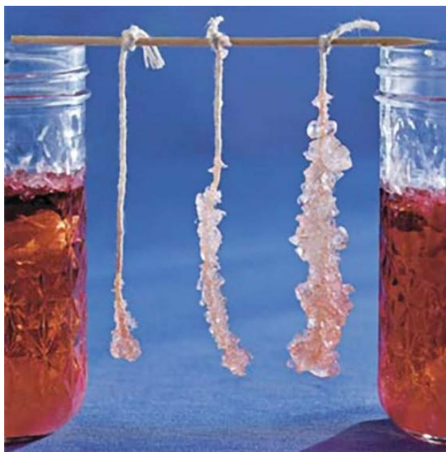
Fig. 17.15 Rock candy. Immersed strings serve as nucleation sites for sugar crystal growth. The sugar solution is first heated; then, as the solution cools, the crystals form.
