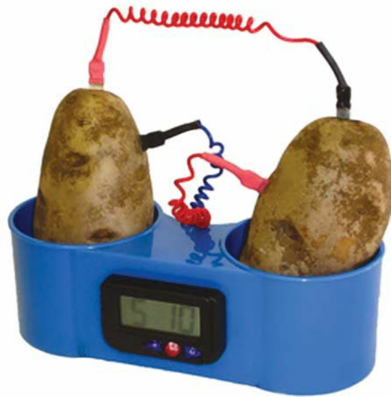
Fig. 12.7 The potato battery. Tomatoes work equally well, and if vegetables are out of season, then salt water can do the trick.
