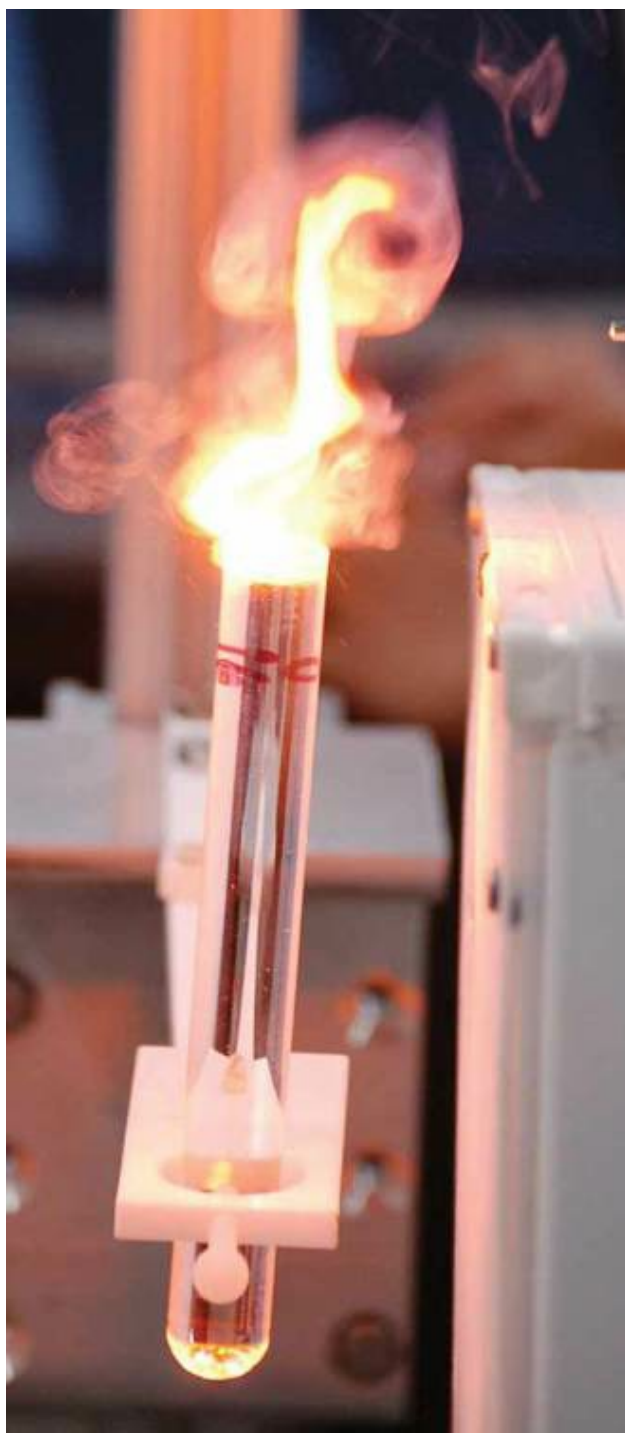
Fig. 7.6 Salt water exposed to electromagnetic energy. The solution catches fire. 3
