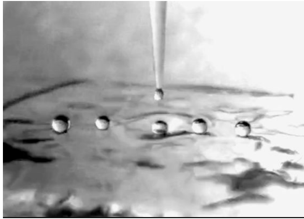
Fig. 16.16 Water droplets falling onto water. Under appropriate conditions, droplets can persist for some time before coalescing with the water below.
